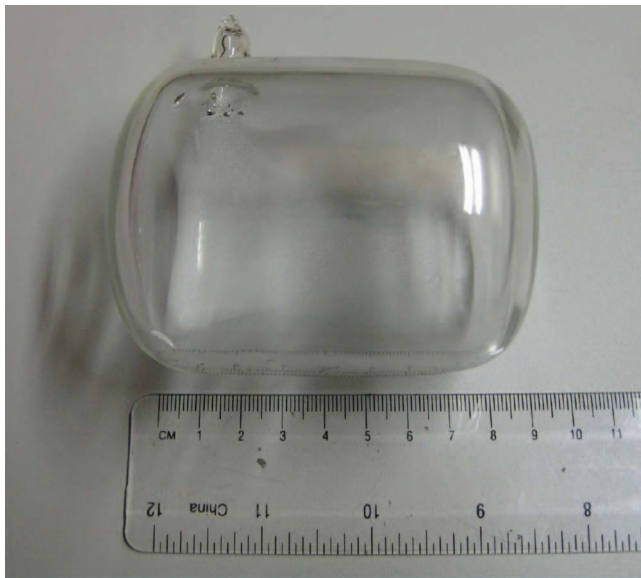
FIG. 1. A typical cylindrical ^3\text{He} cell. The cell is filled with ^3\text{He} and \text{N}_2 gas, as well as alkali metal, usually rubidium (Rb) and potassium (K). The cell described above is not the same but analogous to the cell we used in the present study.
